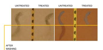
Stain-proofing test carried out on Vicenza stone and terracotta. The untreated section absorbed the grout deep down, which made it difficult to clean after laying.
